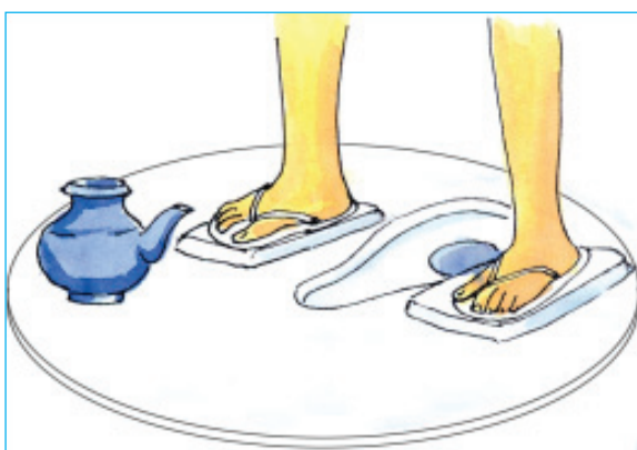
The squat hole should be covered with a fitting lid
